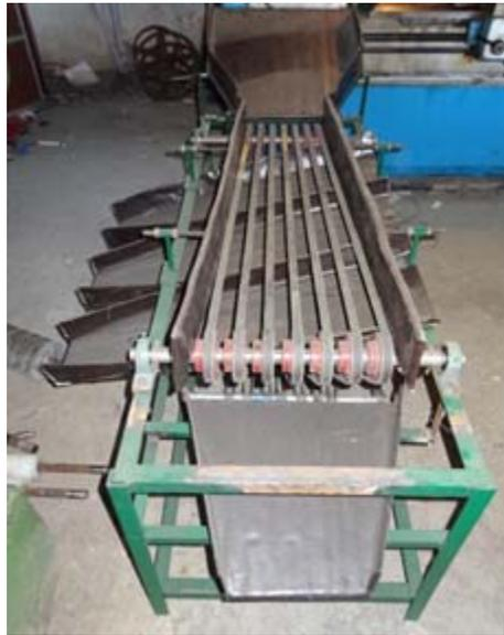
**Figure 1 Expanding pitch type grading machine**
